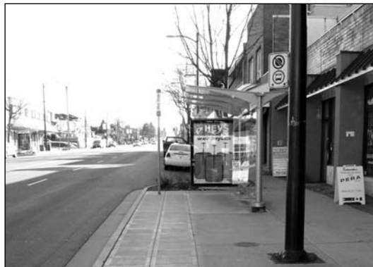
Figure 3-11: Shelter on Bus Bulge and clear of the sidewalk
