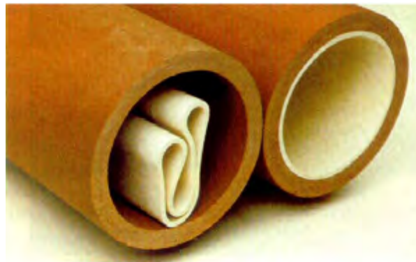
Folded PVC liner for sewer renovation, showing close fit after reversion
