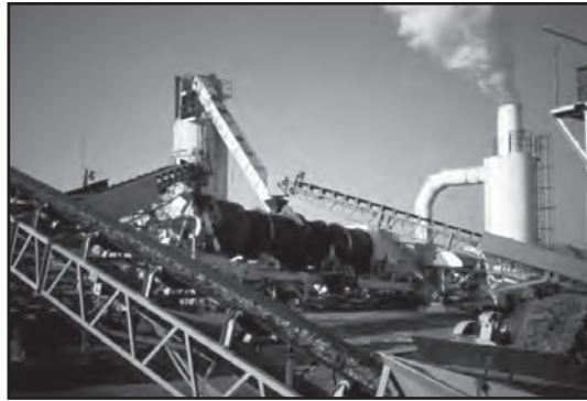
Photo 3-1: Typical parallel flow HMA drum-asphalt plant
