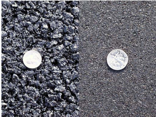
Figure 3–4: Thin open graded hot mix overlay surface on the left; sand mix surface on the right. The diameter of the coins is 18 mm.
