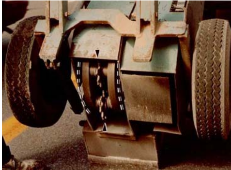
Photograph 3–1: A typical impact router (top) and its carbide-tipped cutters (bottom)
