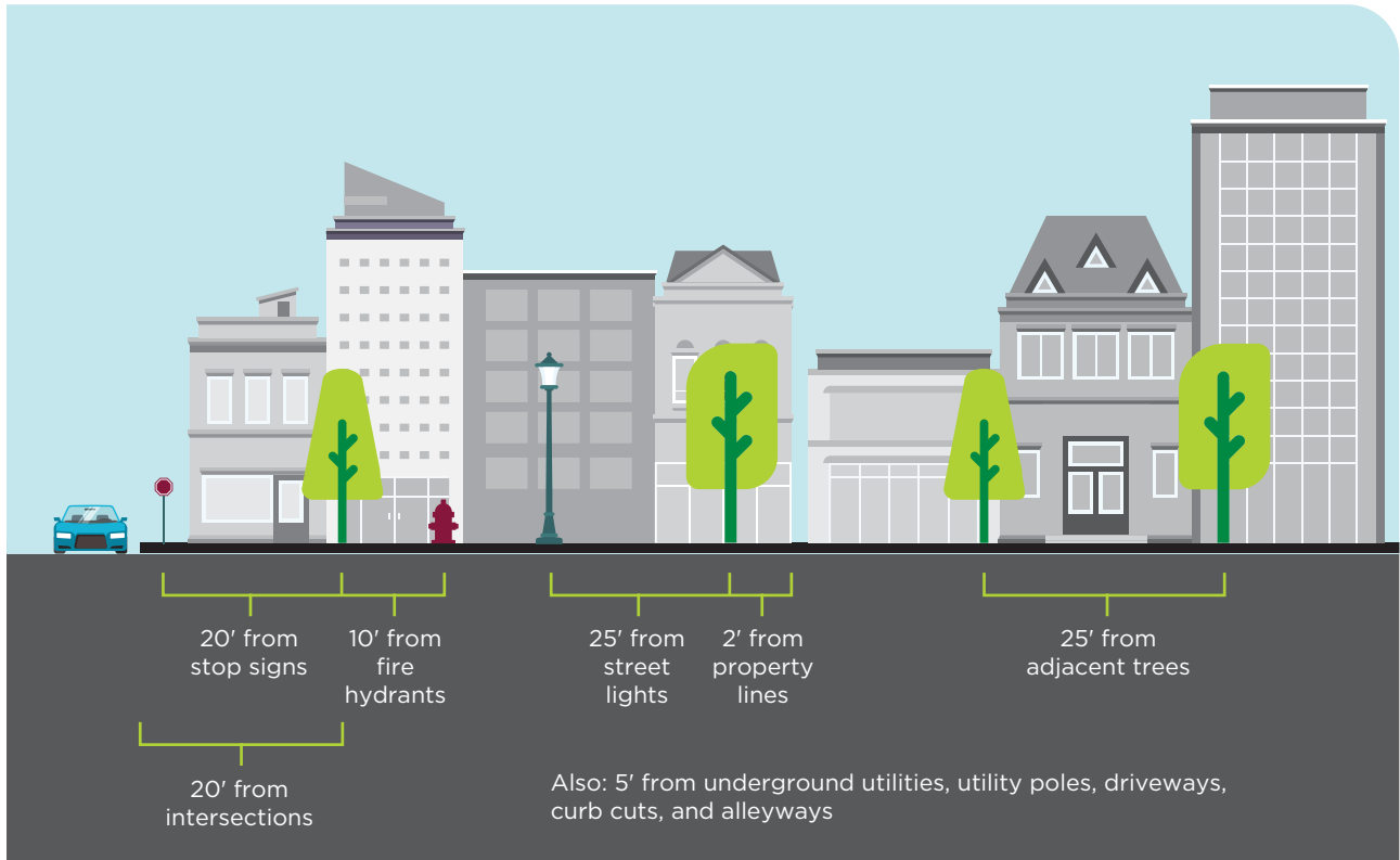
FIGURE 26: EXAMPLE TREE PLANTING DESIGN SHOWING THE DISTANCE REQUIRED BETWEEN NEWLY PLANTED STREET TREES AND EXISTING INFRASTRUCTURE
